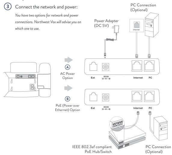
**Note:** If inline power (PoE) is provided, you do not need to connect the power adapter. Make sure the Ethernet cable and hub/switch are PoE compliant.
