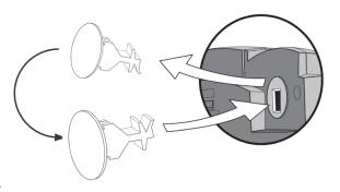
With mounting tab of the base unit facing up, fasten the base stand to wall using wall anchors (not included). When base stand is secured to wall and all cables are connected, snap the SoundPoint® IP-430 into place.
